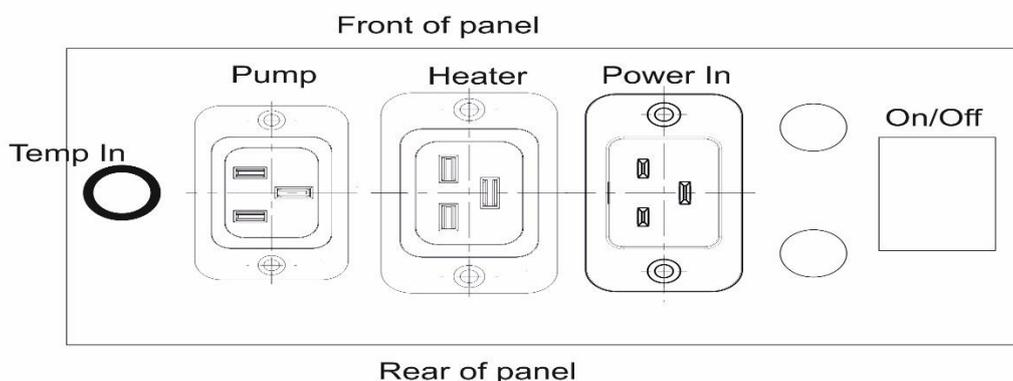
Connect up everything to EINBREW 1V1P and add some water into the vessel. The water level will need to be sufficient to cover the element and to correctly fill the circulation system.
